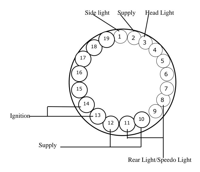
Supply- This is the 'output' of the ammeter.
